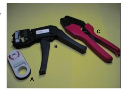
Use tool A to remove 35 mm of the outer sleeving of the cable. This is done by pushing the cable through the small hole in the tool in such a way that the cutter is on the left. Turn the tool in direction MIN (anti-clockwise) a couple of times, the pull off the outer sleeve.
