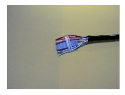
Press the plastic part as far towards the cable as possible. The wires must still be paralell.
