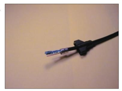
Unwind the twisted pairs. Remove the 3 screen foils. Use a small sharp tool, e.g. a small screwdriver to 'tear' the foil. Tear the outside. This makes it easy to remove the foil with your fingers.
